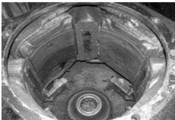
**Gambar 3.** Stator traksi motor
